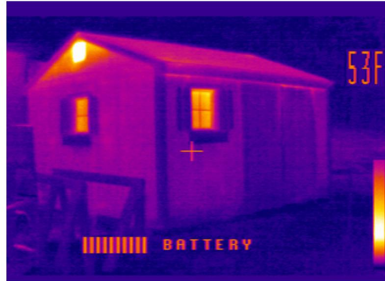
Infra red scanning is helpful in locating air gaps and insulation deficiencies in the envelope and to help develop an overall strategy to air seal and insulate them.
