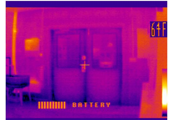
Garage door most significant contributor to air leakage. As they do not use this for vehicle storage, removing the door and framing in a 2x6 wall with one large oversized insulated door is recommended.
