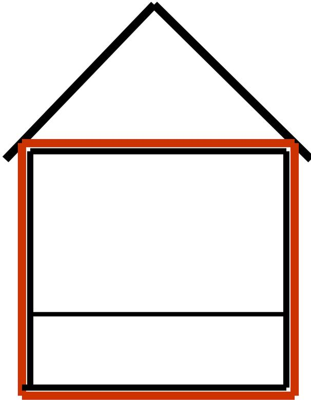
Heating equipment is supposed to be sized to be able to replace all the heat lost thorough the envelope in one hour during one of the coldest winter temps. The more effective the envelope performs, the less heat is lost – the less heat input is needed and the smaller the equipment!!!! (Or summer A/C units!)
