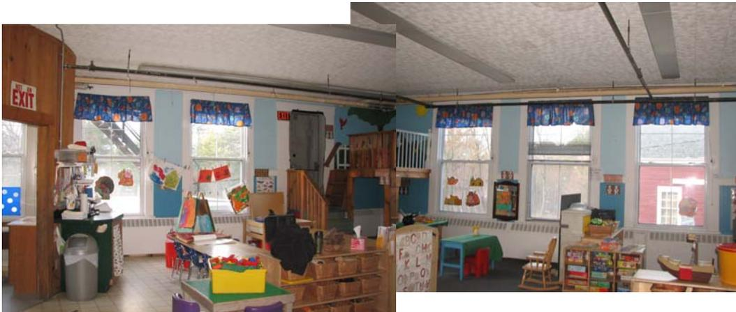
Masonry walls appear uninsulated. Windows are all double pane but of several varieties and fairly 'air leaky'. Each room has an outside exit, which also leak air. Radiating baseboards generally surround each room in order to make up for these high heat loss conditions.
