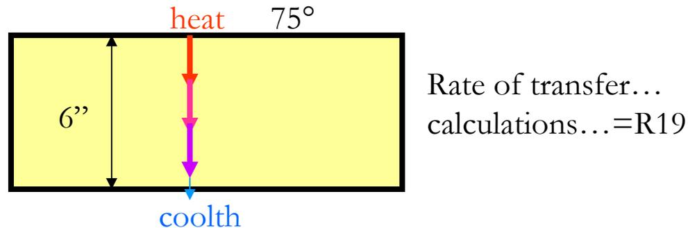
The insulation is in direct contact with a continuous and effective air barrier on all six sides – experiencing no wind or air flow or fluctuations in temperature. And this is how the R19 stamp gets on all 6" fiberglass rolls.
